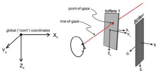
The data reported by *ET3Space* includes head position and orientation, position of the eye and direction of the gaze vector in environment ("room") coordinates, identification of the surface being viewed, the coordinates of the gaze point on that surface, and pupil diameter. Data are displayed in real-time, can be streamed to external devices in real-time via Local Area Network, and can be recorded on a digital data file.
